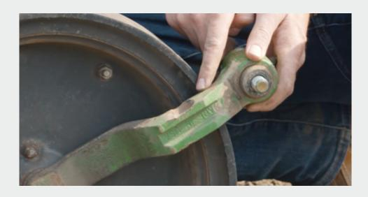
It's very important to check the following components of the depth adjustment linkage for wear:
